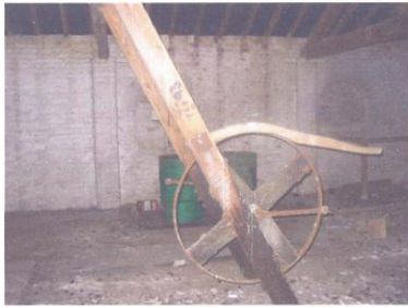
First floor pulley wheel. Note the wooden hand operated brake.
